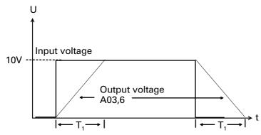
Time constants with unchanged integration capacitor (C9 =  $1\mu$ F):
